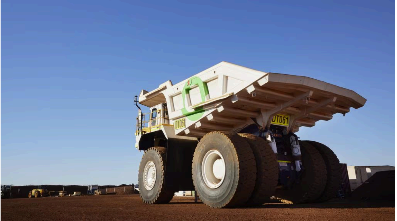
One of Fortescue's battery-operated haul trucks.
