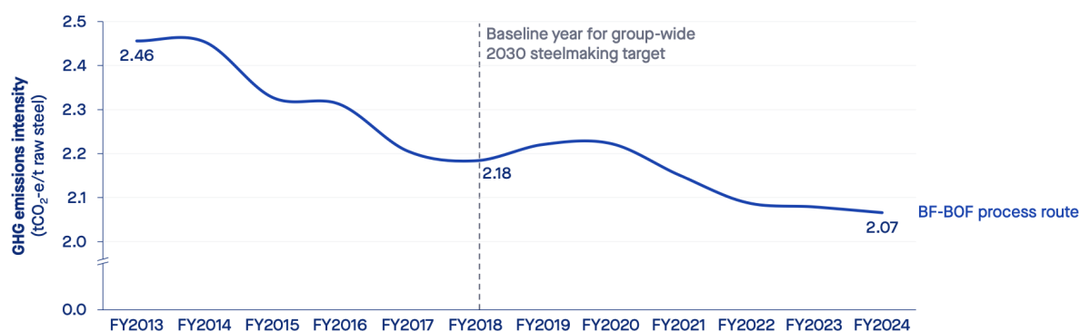
Figure 3.5: BlueScope's Port Kembla BF-BOF Emissions Profile
